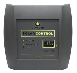
The purpose of the LSP-SC1 controller is to control a simple solar thermal system, which consists of a solar collector, storage tank and a pump. Comparing the temperatures of the collector and of the storage tank, this device controls the pump and makes sure that the entire system is safe and highly efficient. It was designed for easy installation and usage.
