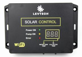
The purpose of the LSP-SC2-WIFI controller is to control a solar collector system consisting of a solar collector and a hot water storage tank. By comparing the collector and tank temperatures, the device controls the pump and assures the user that the system is operating safely and efficiently. The controller is configured using our smartphone or a laptop with which we connect to the device via WiFi.
