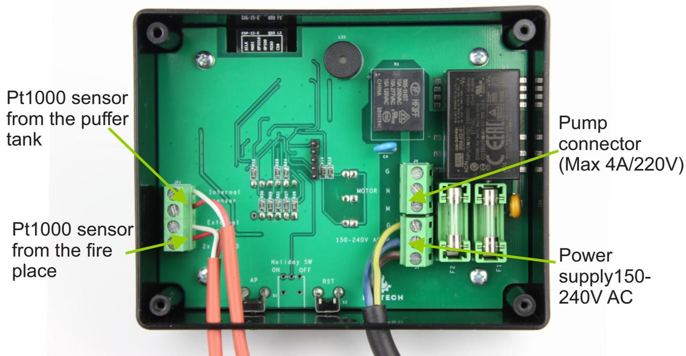
By default, the two temperature sensors and the power cable are connected to the controller. Before use, it is only necessary to connect the motor wires properly. If the wires of one of the sensors need to be extended, it is justified to dismantle, splice and reassemble them. The sensors can be extended to a length of up to 300 m without affecting the accuracy of the measurement.
