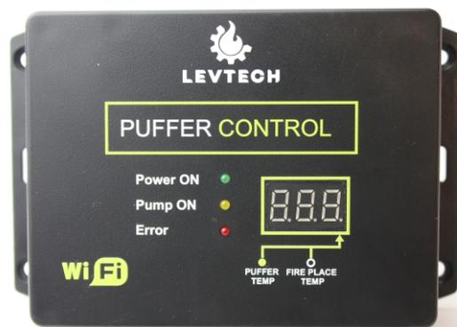
The purpose of the LSP-PC1-WiFi controller is to effectively control the heating of the puffer tank. The controller has two temperature sensors and controls a pump. Based on the temperatures measured in the fire place and the puffer tank, as well as the set parameters, it controls the pump and assures the user that the system works safely and efficiently. The controller is configured using our smartphone or a laptop connected via WiFi.
